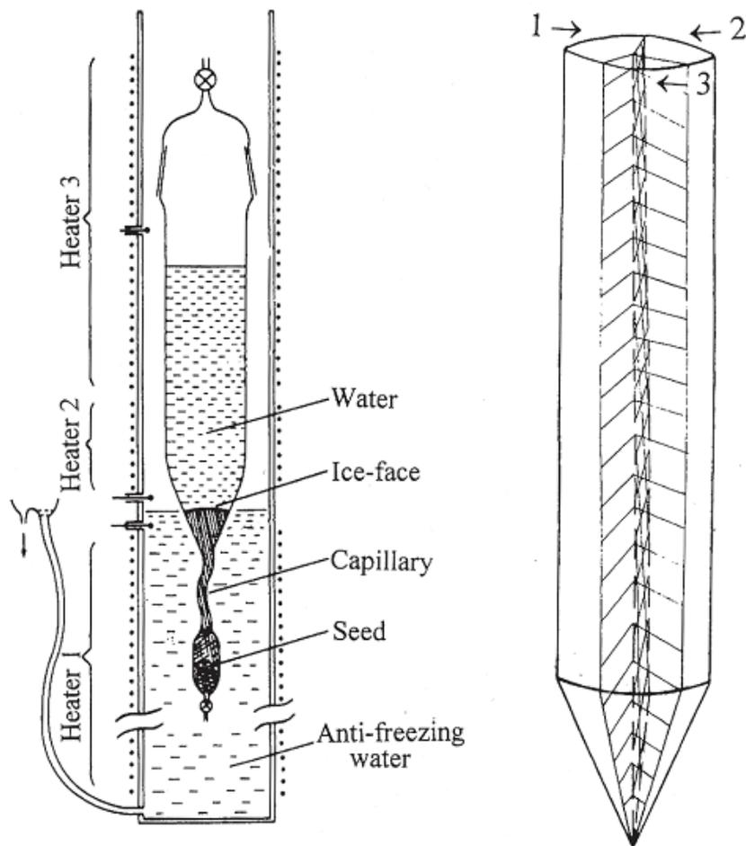
Figure 3. The left diagram shows a schematic illustration of the Bridgman method of crystal growth system<sup>23</sup>. The right diagram is a crystal of ice Ih produced by the system (using the  $I_E$  water). In most cases, we were able to produce ice crystals as easily as the high purity normal water. However, for the  $I_E$  water labeled with Ds-PB provided by ATG, we obtained 2-3 pieces of single crystals, after a number of attempts as shown in the right diagram.
