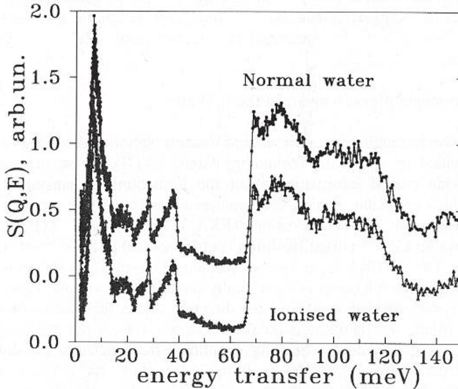
Figure 1. A plot of Inelastic Incoherent Neutron Scattering spectra of the  $I_E$  water and normal water measured on TFXA in the energy transfer region below 140 meV at temperature of 15K. The data show that difference between the two spectra is less than the experimental error.
